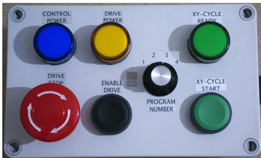
Component setup for a dual axis marking system with TMC-200-VE, inkjet, XY-linear portal robot and operator box (picture below) as user interface
