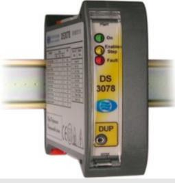
... featuring an industrial quality motion controller/drive type LAM DS3078 with on board application software TMC-200 ...
