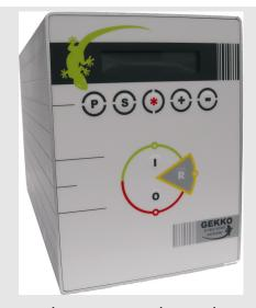
... combining an industrial quality high speed motion controller/stepper drive with a user friendly HMI interface ...
